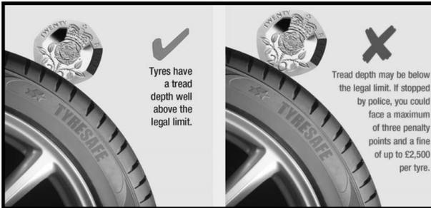
The 20p test – check your tyre tread with a 20p by placing it into the main groove of your tyre. The outer band of the 20p coin should be obscured when it is inserted. TyreSafe have produced a great example of this:
